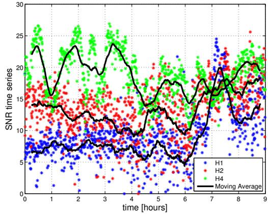
Figure 4. Time series of SNR for transmissions from T2 during experiment B. Moving averages over 50 samples are provided as a solid black line.
