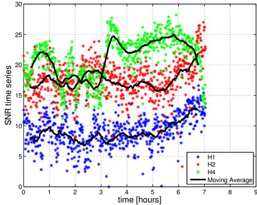
Figure 3. Time series of SNR for transmissions from T2 during experiment A. Moving averages over 50 samples are provided as a solid black line.
