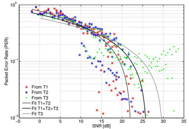
Figure 2. Log-scale scatterplot of PER as a function of SNR for varying transmitter and all receivers. Linear fits of the joint scatterplot of all transmitters as compared to the joint scatterplot of T1 and T2, as well as the scatterplot of T3, are also provided.
