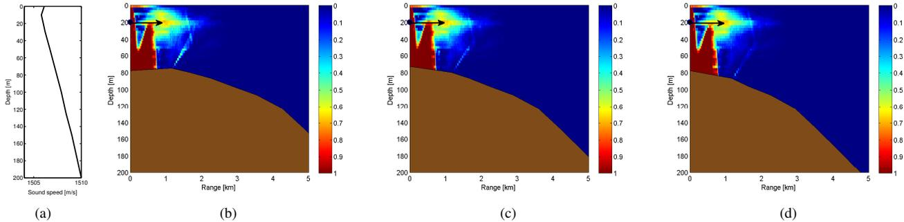
Figure 2. Example of next hop choices in a shallow water scenario in winter. (a) sound speed profile; (b)–(d) 1<sup>st</sup> to 3<sup>rd</sup> hop. Red hues correspond to a higher probability that the received SNR exceeds a threshold of 20 dB.
