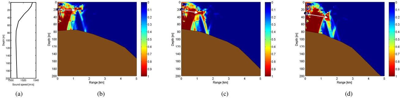
Figure 1. Example of next hop choices in a shallow water scenario in summer. (a) sound speed profile; (b)–(d) 1<sup>st</sup> to 3<sup>rd</sup> hop. Red hues correspond to a higher probability that the received SNR exceeds a threshold of 20 dB.
