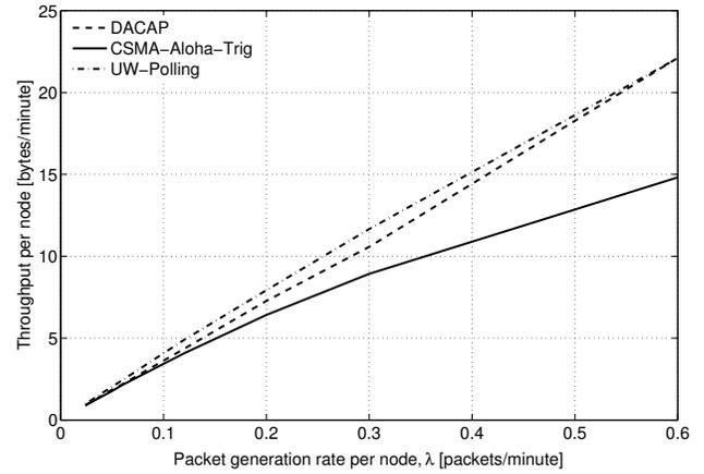
Figure 5. Throughput as a function of the packet generation rate,  $\lambda$  in packets per minute per node. The source power level is 150 dB re  $\mu$ Pa.
