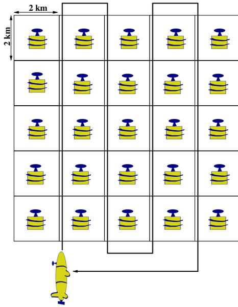
Figure 3. Topology of the network and trajectory of the AUV.
