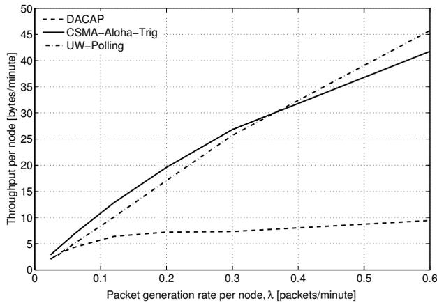
Figure 9. Throughput as a function of the packet generation rate,  $\lambda$  in packets per minute per node. The source power level is 190 dB re  $\mu\text{Pa}$ .
