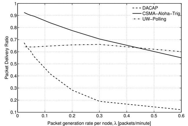
Figure 10. Packet delivery ratio as a function of the packet generation rate,  $\lambda$  in packets per minute per node. The source power level is 190 dB re  $\mu\text{Pa}$ .
