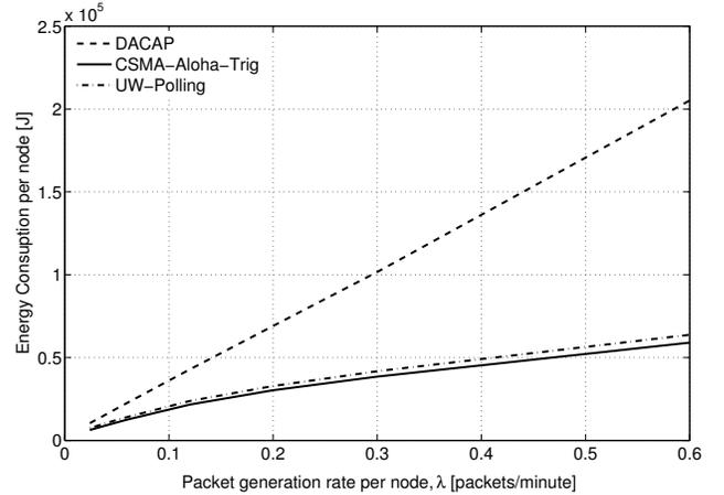
Figure 8. Energy consumption per node as a function of the packet generation rate,  $\lambda$  in packets per minute per node. The source power level is 150 dB re  $\mu\text{Pa}$ .
