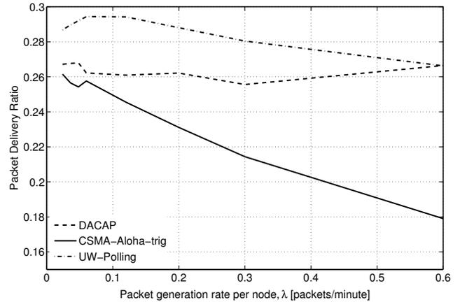
Figure 6. Packet delivery ratio as a function of the packet generation rate,  $\lambda$  in packets per minute per node. The source power level is 150 dB re  $\mu$ Pa.
