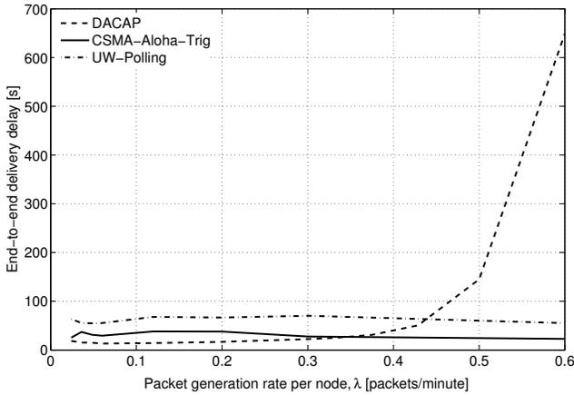
Figure 7. End-to-end delivery delay as a function of the packet generation rate per node,  $\lambda$  in packets per minute per node. The source power level is 150 dB re  $\mu\text{Pa}$ .
