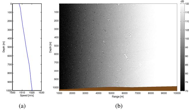
Figure 4. Simulation scenario at (41.90°N, 17.51°E): (a) Monthly averaged January SSP from [12]; (b) channel power attenuation obtained using Bellhop (coherent mode) at a frequency of 25 kHz. The mild increase of the SSP for increasing depth translates into a relatively uniform propagation pattern.
