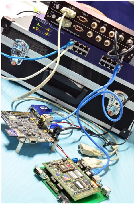
Fig. 2. Hardware prepared for a laboratory test to be conducted with the WHOI Micro-Modem Software Development Board (the black box on the upper right corner of the picture).
