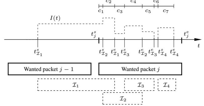
**Figure 1: Chunk interference model implemented in DESERT Underwater.**
