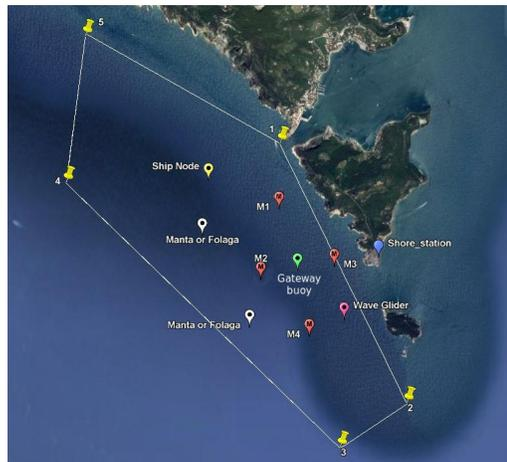
Fig. 10. A comprehensive snapshot of the network deployment during the CommsNet'13 sea trials in La Spezia, Italy. The yellow pins delimit the operational area. The network includes bottom-mounted nodes, a ship node, an acoustic/radio gateway buoy, two autonomous underwater vehicles and one autonomous surface system.
