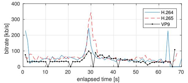
Fig. 6. Received bitrate during the video stream, with H.264 (solid blue line), H.265 (red dashed line) and VP9 (black line with point marks) codecs.
