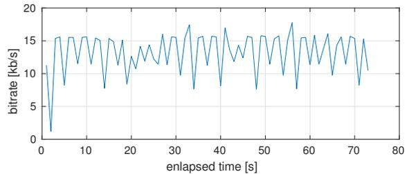
Fig. 7. Received bitrate during the low quality video stream via acoustics.
