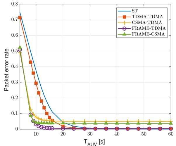
Fig. 7. Packet error rate of monitoring packets.
