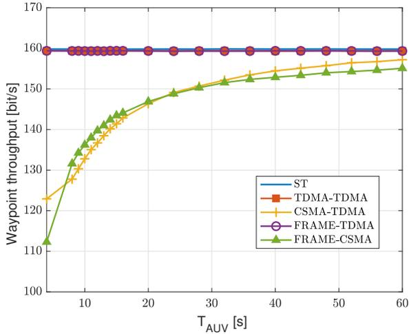
Fig. 3. Average throughput received by the AUV.
