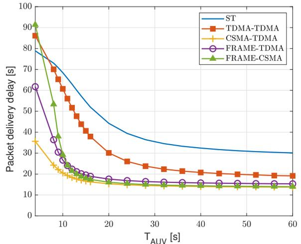
Fig. 8. Average packet delivery delay of the monitoring traffic.
